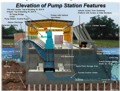
gates and pumps stormwater from each canal back into the lake. The pumps have a combined capacity of 24,300 cubic feet per second.
