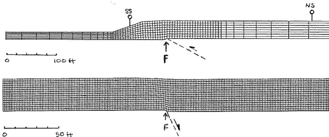
**Figure 23** Finite element meshes representing soil overlying shallow thrust fault rupture (Section R-R' shown at top) and hanging-wall bending moment normal fault rupture (Section X-X' for 65° dipping normal fault shown at bottom). Meshes drawn with scale of 10 ft = 3.05 m. “F” denotes tip of bedrock fault, and “SS” and “NS” denote south and north setbacks, respectively.
