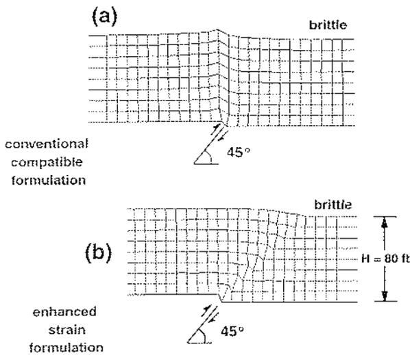
**Figure 21** Improved performance of enhanced strain element compared to conventional compatible formulated element for modeling response of saturated clay to 45 degree reverse fault displacement (after Lazarte 1996).
