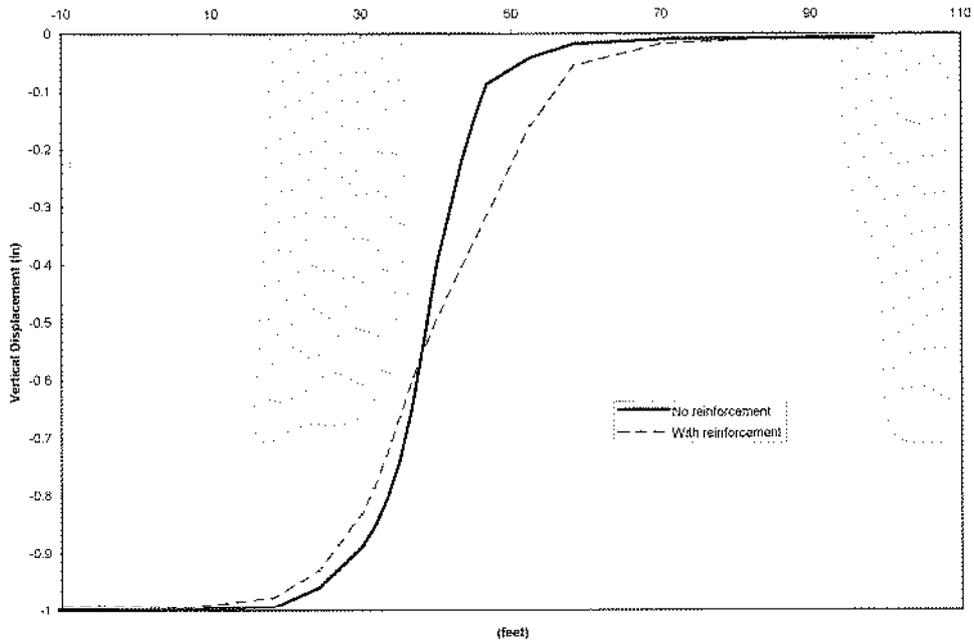
**Figure 25** Finite element results showing beneficial effect of installing two layers of geogrids into compacted fill. The underlying differential fault offset is spread across a wider zone with reinforced fill, thereby reducing Hazards B and C. Case shown is for 6 m-high reinforced and unreinforced fill composed of Soil B for 2.8 cm of displacement across a normal fault dipping at 65 degrees (1.0 inch = 2.5 cm, and 1.0 feet = 0.305 m).
