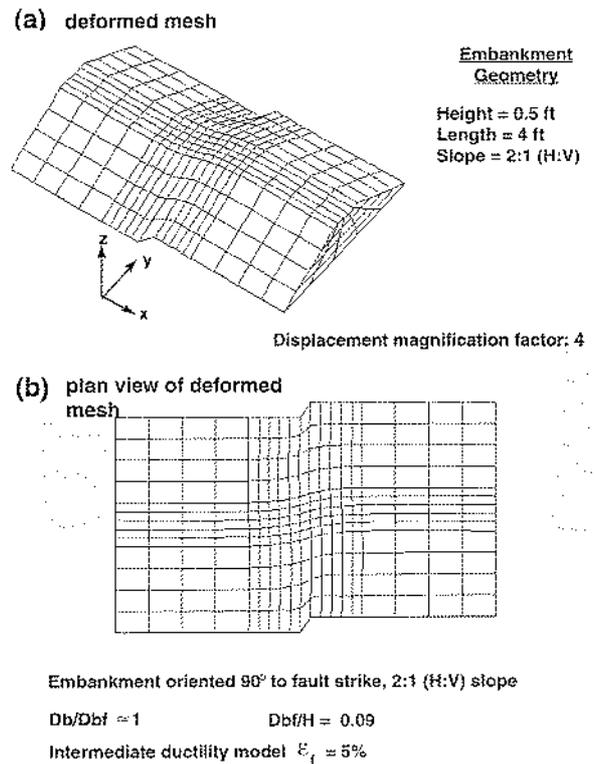
**Figure 22** Three-dimensional finite element analysis of physical model experiment investigating the response of saturated clay embankment to foundation strike-slip fault movement (after Lazarte 1996).
