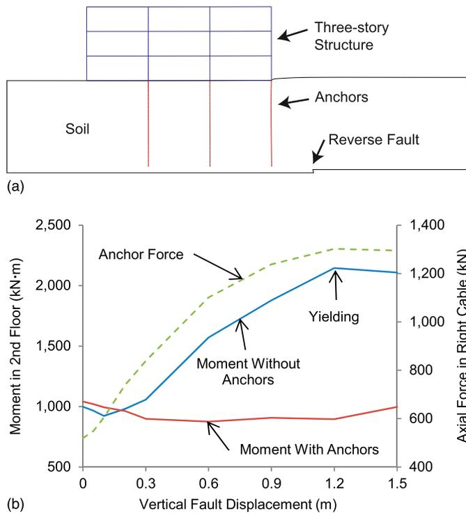
**Fig. 11.** Comparison of building response with and without ground anchors: (a) model geometry with anchors; (b) loads induced in the structure are significantly decreased when the anchors are used (reverse fault, 60° dip, 15-m-thick soil deposit, 2.0 m of previous vertical fault movement,  $N_{1,60} = 22$ ,  $K_o = 0.45$ , 0.45-m-thick mat foundation, 1,500-kN anchor capacity, 500-kN pretensioning, and 5-m anchor spacing)
