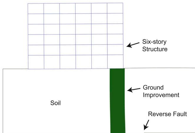
**Fig. 9.** Ground improvement by densification of the soil beneath a structure results in estimated slight damage compared with moderate to severe damage according to the definitions in Boscardin and Cording (1989) for this representative situation [reverse fault, 60° dip, 25-m-thick soil deposit, 0.6 m of vertical fault movement, no previous fault movement,  $N_{1,60} = 12$  ( $N_{1,60} = 36$  in densified zone),  $K_o = 0.45$ , and 0.45-m-thick mat foundation]
