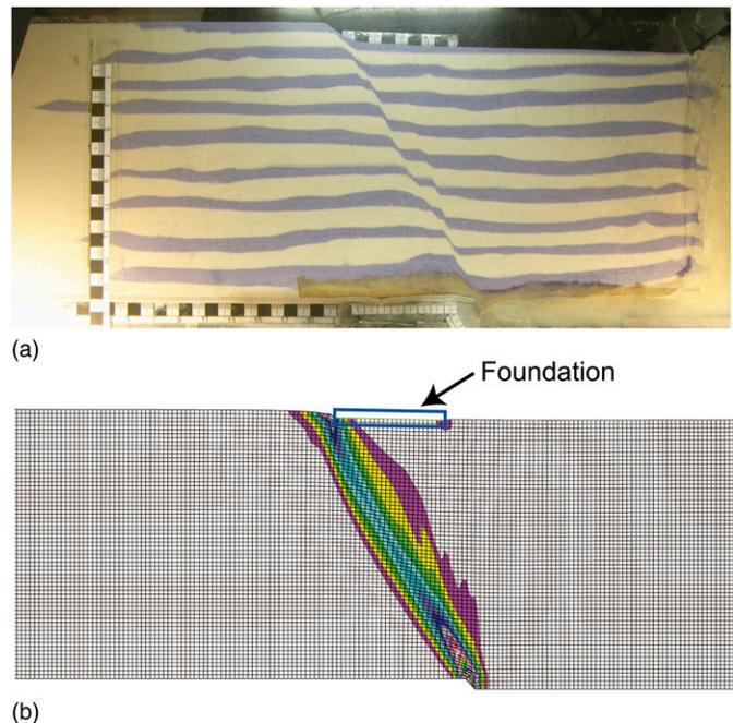
**Fig. 1.** Validation of the numerical model with centrifuge Test 14 from Bransby et al. (2008b): (a) photograph of the centrifuge experiment; (b) deformed mesh and shear strain contours for the numerical model (normal fault, 60° dip, 2.0 m of vertical fault movement, 24.5-m-thick soil deposit,  $N_{1,60} = 23$ , and  $K_o = 0.45$ ); the lateral extent of the finite-element mesh on the left side has been cropped
