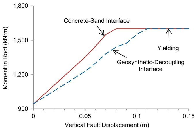
**Fig. 8.** Comparison of building performance with and without a decoupling geosynthetic slip layer (normal fault,  $30^\circ$  dip, 15-m-thick soil deposit, no previous fault movement,  $N_{1,60} = 22$ ,  $K_o = 0.45$ , 0.45-m-thick mat foundation, and  $11^\circ$  interface friction compared with the full friction angle of the sand)
