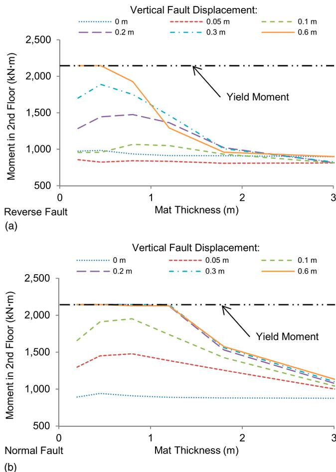
**Fig. 6.** Comparison of building performance with mat foundations of varying thickness: (a) reverse fault; (b) normal fault ( $60^\circ$  dip, 15-m-thick soil deposit, 2.0 m of previous vertical fault movement,  $N_{1,60} = 22$ , and  $K_o = 0.45$ ); the relevant problem geometry is provided in Fig. 3(a), and the maximum moment in the reverse fault case decreases for very small fault movements because the location of maximum moment is shifting
