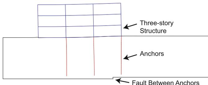
**Fig. 12.** Structure can be more damaged with anchors installed than if no anchors were present if the fault ruptures between anchors, thus only tying part of the building down
