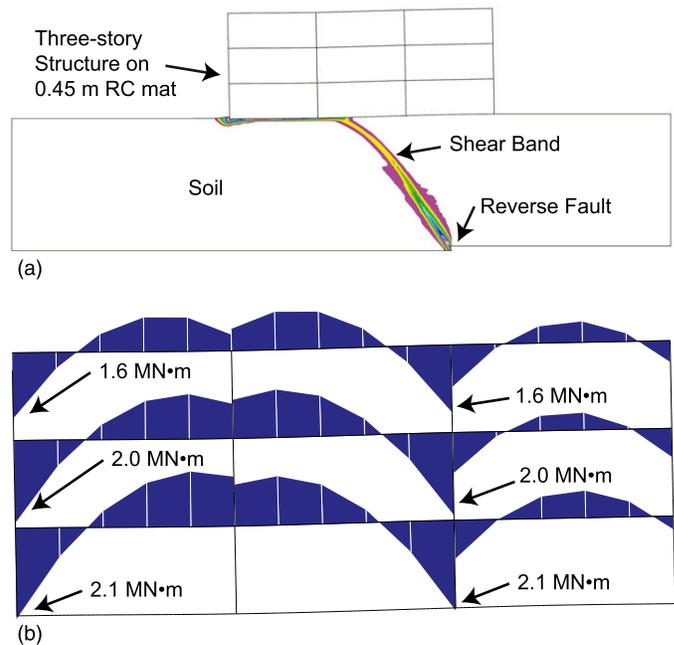
**Fig. 3.** (a) Representative soil response because of underlying reverse fault rupture of 0.6 m in the vertical direction (shear strain contours shown;  $0.2 \times 0.2$ -m mesh size used); (b) representative moments induced in the beams by fault rupture (the noted maximum values are where yielding is occurring)
