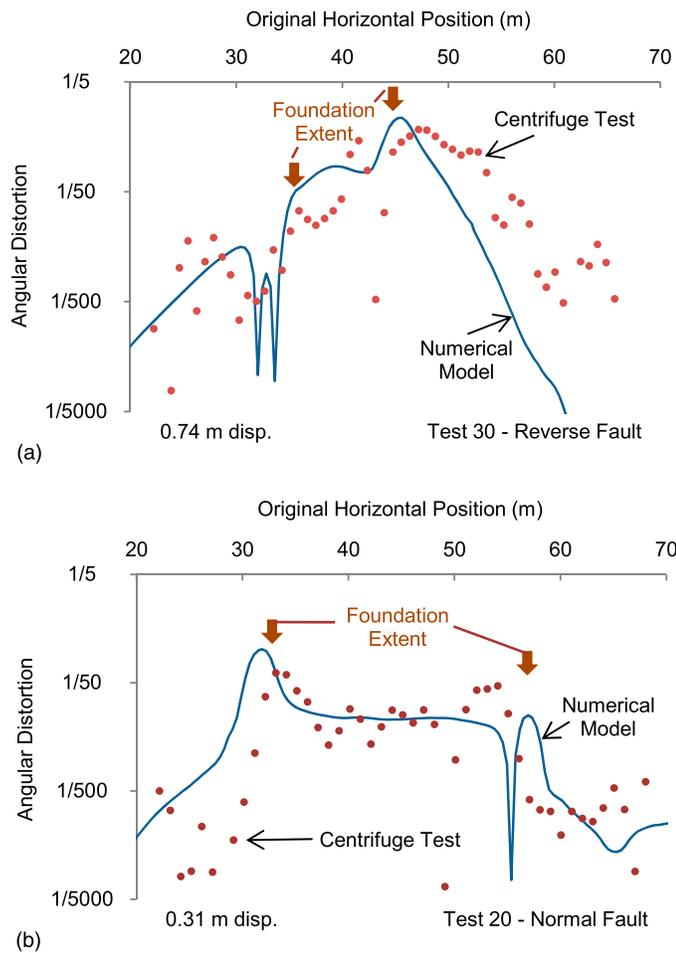
**Fig. 2.** Comparison between the centrifuge test (Bransby et al. 2008a, b) and numerical results for (a) centrifuge Test 30 (reverse fault,  $60^\circ$  dip, 15-m-thick soil deposit, 0.74 m of vertical fault movement,  $N_{1,60} = 31$ ,  $K_o = 0.45$ , 10-m-wide mat, and 37-kPa mat load); (b) centrifuge Test 20 (normal fault,  $60^\circ$  dip, 25-m-thick soil deposit, 0.31 m of vertical fault movement,  $N_{1,60} = 19$ ,  $K_o = 0.45$ , 25-m-wide mat, and 84-kPa mat load)
